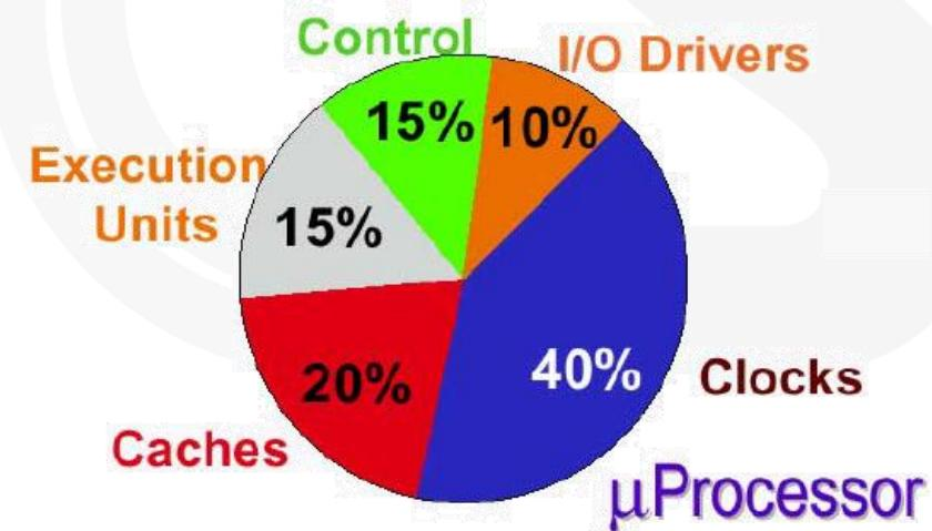
Possible power partitioning of a microprocessor (not general!!!!)
