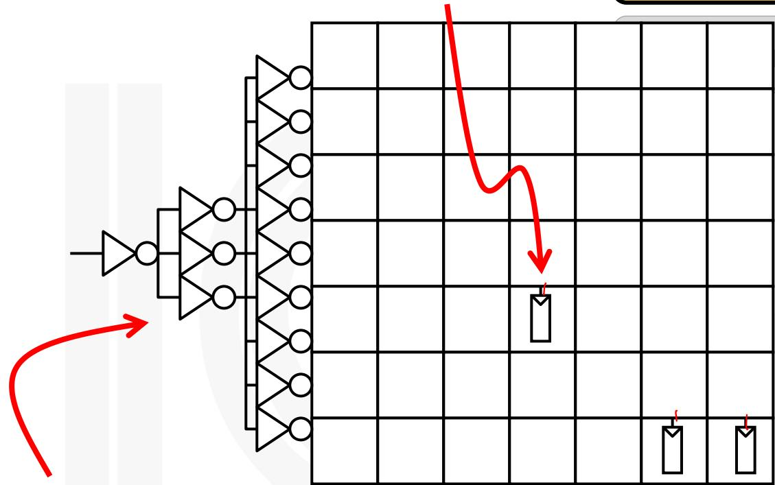
Clock driver tree spans height of chip
