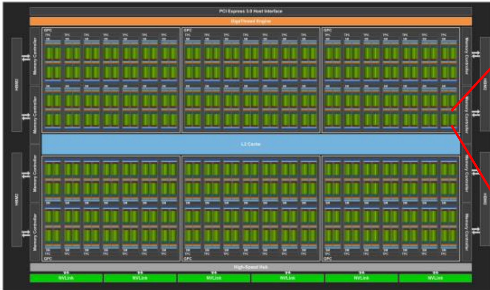
Volta GV100 Full GPU with 84 SM Units
