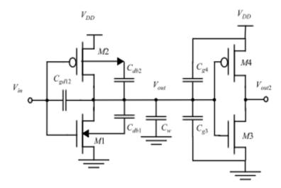
All capacitances are lumped together into one single output capacitance:
