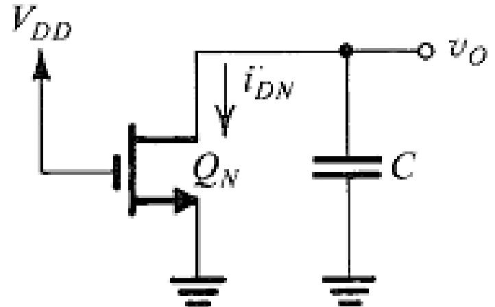
$$I_{Dn} = \frac{k_n}{2} (V_{GSn} - V_{Tn})^2 (1 + \lambda V_{DS}) \approx \frac{k_n}{2} (V_{in} - V_{Tn})^2$$
