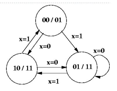
Mealy machines have an output that is determined by the previous state and the input:
