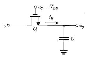
$\mu_n C_{ox} = 50 \mu; \ \mu_p C_{ox} = 20 \mu; \ |V_{T0}| = 1V;$   $\gamma = 0.5 V^{1/2}; \ \Phi_F = -0.3 V; \ \lambda = 0.1$  $V_{DD} = 5 V; \ (W/L)_n = 4 \mu/2 \mu; \ C_L = 50 fF$
