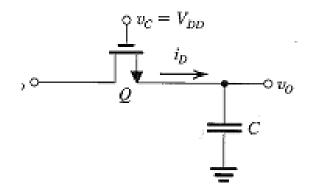
$$t_{pLH} = C_L \frac{V_{DD}/2 - 0}{I_{Avg}} = 50f \cdot \frac{2.5}{632\mu} = 198p \sec$$
