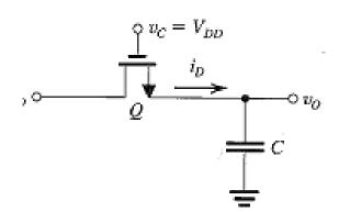
The most important aspect here is that the Source and Drain change sides!
