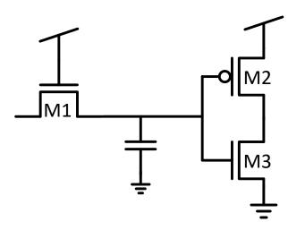
$$\mu_{n}C_{ox} = 50\mu; \ \mu_{p}C_{ox} = 20\mu; \ |V_{T0}| = 1V;$$
