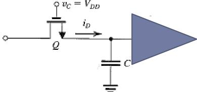
$\mu_{n}C_{ox} = 50\mu; \ \mu_{p}C_{ox} = 20\mu; \ |V_{T0}| = 1V;$   $\gamma = 0.5V^{1/2}; \ \Phi_{F} = -0.3V; \ \lambda = 0.1$   $V_{DD} = 5V; \ (W/L)_{n} = 4\mu/2\mu; \ C_{L} = 50fF$   $INV: (W/L)_{p} = 2.5(W/L)_{n} = 10\mu/2\mu;$
