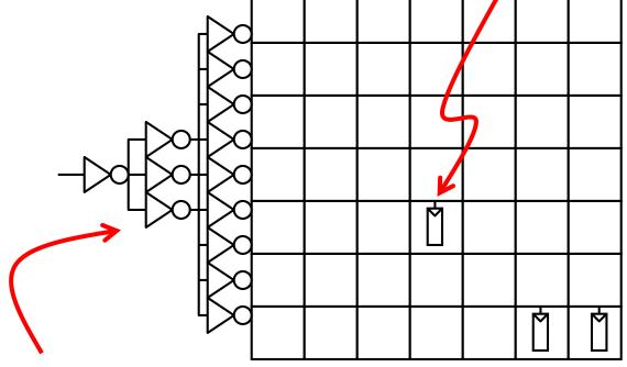
Clock driver tree spans height of chip Internal levels shorted together
