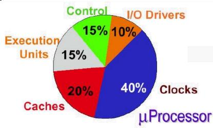
Possible power partitioning of a microprocessor (not general!!!)
