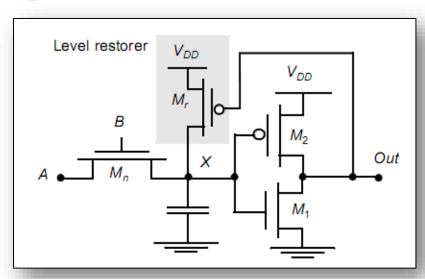
This means we need careful Ratioed Sizing to make the circuit work properly.
