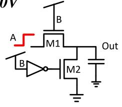
□ Since *M2* is cut-off, we can just remove it from our equivalent model:
