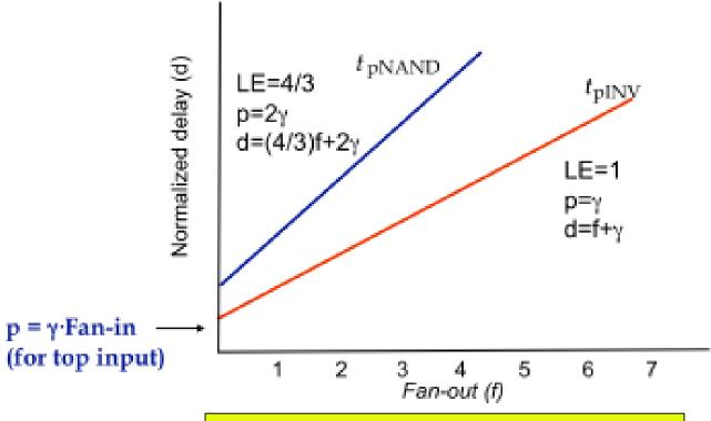
$$p \triangleq \frac{R_{gate}}{R_{inv}} \frac{C_{d,gate}}{C_{d,inv}} \qquad LE \triangleq \frac{R_{gate}}{R_{inv}} \frac{C_{g,gate}}{C_{g,inv}}$$
